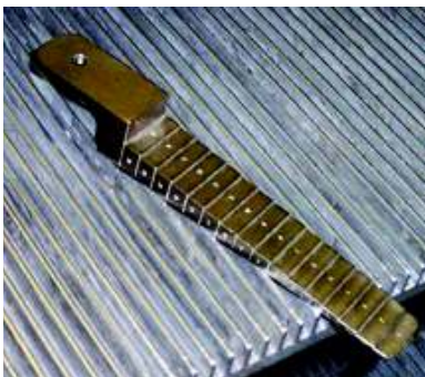
Figure 1.2 Stepped gauge used to check gaps.
